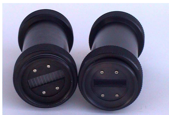
Figure 3 Lenslet array and mount for initial 10 and 40-element sensors.
